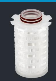
BorsoPTFE-JM junior cartridges are manufactured with a zPTFE membrane with a reduced resistance to flow while fully retaining bacteria. The cartridges are highly resistant to thermal stress during steam sterilization. A multitude of adaptor options are available for easy retrofitting into existing housings.
