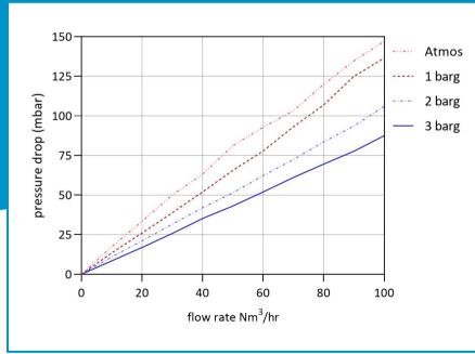
Air flow vs pressure drop at various pressures for a 5 inch BorsoPTFE-JM, 0.2 µm zPTFE membrane junior cartridge
