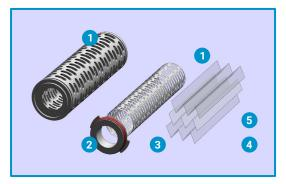
Finite Element Analysis optimised polypropylene cage (1)
