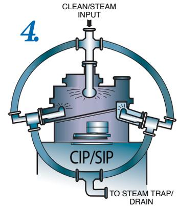
**NO-GAP DESIGN ALLOWS FULL CIP / SIP CAPABILITY.**
